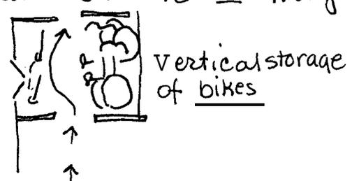
④ place brackets on walls - OR ceiling and floor. to hold wheels of bikes. Top bracket needs to hold front wheels from flopping
