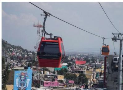
**Gondola** - Also known as aerial tramways, these systems are a type of cable car pioneered for ski resorts, but have been deployed in urbanized areas to avoid the issues related to surface infrastructure. Passenger capacity can range from four passengers up to 100 per car, and the systems will typically have only two cars and two stops.
