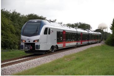
**Light Rail/Electric Multiple Unit – Light Rail/EMUs** are popular on commuter and suburban rail networks around the world due to their fast acceleration and pollution-free operation. Being quieter than diesel multiple units locomotive hauled trains, EMUs require no separate locomotive, as electric traction motors are incorporated within one or a number of the carriages, and are compatible with freight rail.
