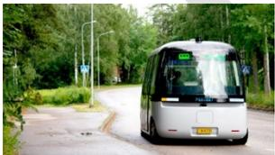
**Micro-shuttles** – Smaller passenger autonomous vehicles (12-15 persons operating at low speed and fixed routes. Manufacturers have been developing fully autonomous versions, with several deployed in the United States and California.
