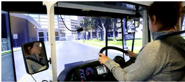
Redesigned MB-1000 and MB-2000 bus simulators (new vehicle dynamics, steering system, motion platform, fully upgraded realistic virtual training world "Safety City," electric bus training features, and upgraded VITALS training assessment tool). 2020
