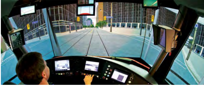
Light rail vehicle simulator using a replica Bombardier cab delivered to Toronto Transit (TTC). 2013
